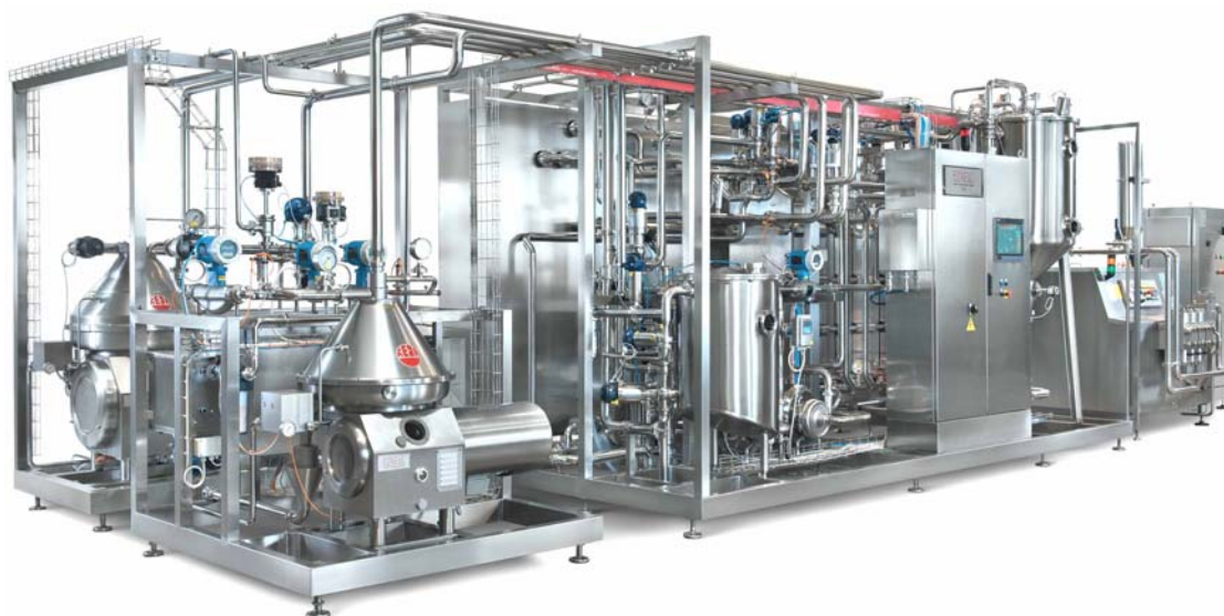
Example of REDA line for "ESL Milk" of 10,000 L/h with milk separator, bacteria separator and in-line automatic standardizer
