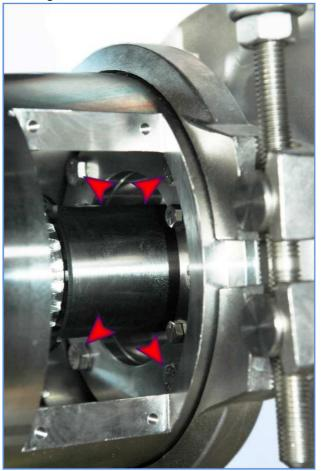
6. Partially tighten the 4 screws of the seal bushing;
