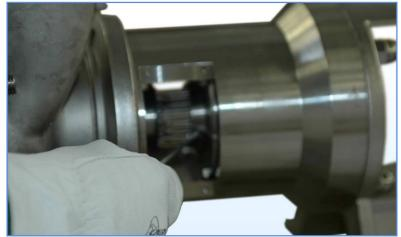
4. To facilitate alignment of the drive coupling manually rotate the shaft on the idle side;
