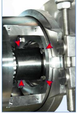
7. Correctly align the bushing flange and tighten the 4 screws;
