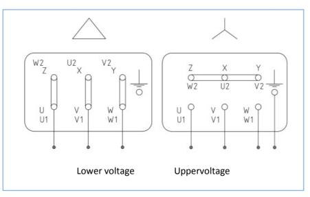
During the motor starting phase, current absorption increases for a very short time to 5-6 times the nominal value, if the mains are unable to withstand this absorption peak, star-triangle starters or other systems must be used (e.g. auto-transformer).
