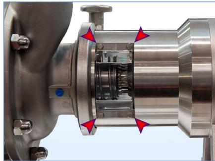
4. Loosen the 6 bolts from the head, idle side;
